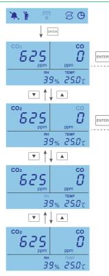
Calibrate CO2: when CO2 is blinking, press ENTER to start calibration, wait for 3-5 minutes till CO2 reading is stable, press ENTER to finish calibration.
